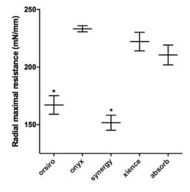
**FIGURE 4** Radial maximal resistance (mN/mm). \**P* < 0.001 for Orsiro and Synergy vs Absorb, resolute Onyx, and Xience Alpine
