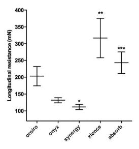
**FIGURE 5** Longitudinal maximal resistance (mN). \*P < 0.001 for Synergy vs Orsiro, Xience Alpine, and Absorb, \*\*P < 0.001 for Xience Alpine vs all other devices; \*\*\*P < 0.001 for Absorb vs resolute Onyx, Xience Alpine, and Synergy
