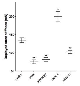
**FIGURE 3** Deployed stent stiffness (mN). \*P < 0.001 for Orsiro and Xience Alpine vs all other devices. \*\*P < 0.001 for Synergy vs Orsiro and Xience Alpine; \*\*\*P < 0.001 for Absorb vs Orsiro, resolute Onyx, and Xience Alpine
