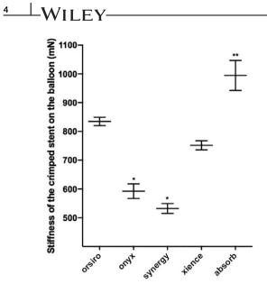
**FIGURE 2** Stiffness of the stent crimped on the balloon (mN). \*P < 0.001 for resolute Onyx and Synergy vs Orsiro and Xience Alpine. \*\*P < 0.01 for Absorb vs all other devices
